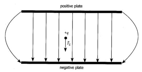
In the region between the plates, the electric field lines are parallel and evenly spaced, indicating that the field has a uniform magnitude and direction throughout.
